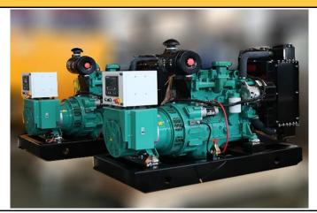
Model:KH-24GF Engine: CUMMINS Alternator: STAMFORD Control Panel: UK DEEPSEA Prime Power:30KVA/24KW Standby Power:33KVA/26.4KW
